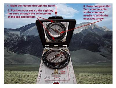
compass needle is lined up in the engraved arrow. Double check to make sure compass is perfectly flat so the compass needle can pivot freely.
